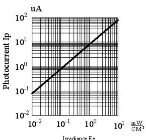
Irradiance Ee Fig6 PHOTOCURRENT VS IRRADIANCE λ =940nm
